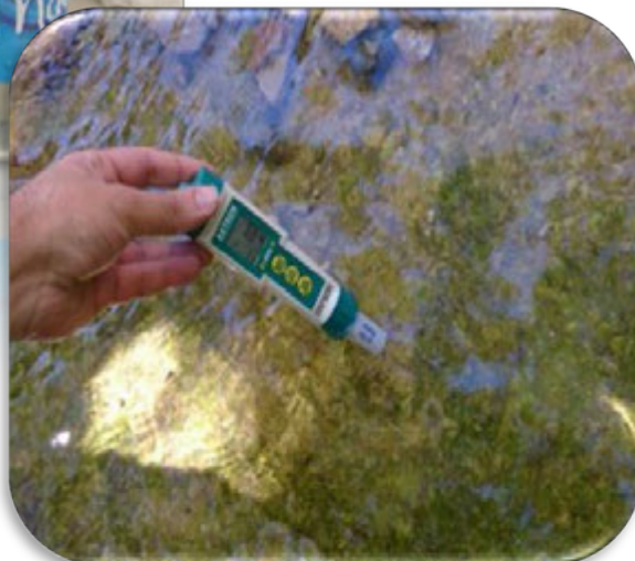
EC400 ExStik Conductivity/TDS/Salinity Meter.
