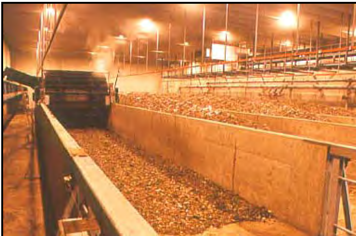
Figure VIII-9. Metro- or channel-type system, showing channels and agitator at left centre
