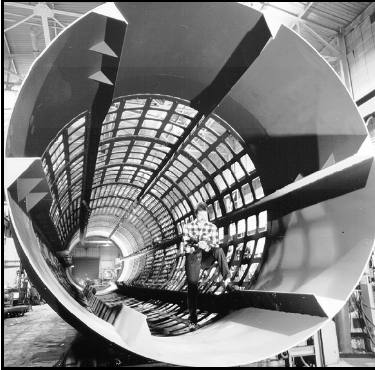
Figure VI-14. End view of a trommel screen
