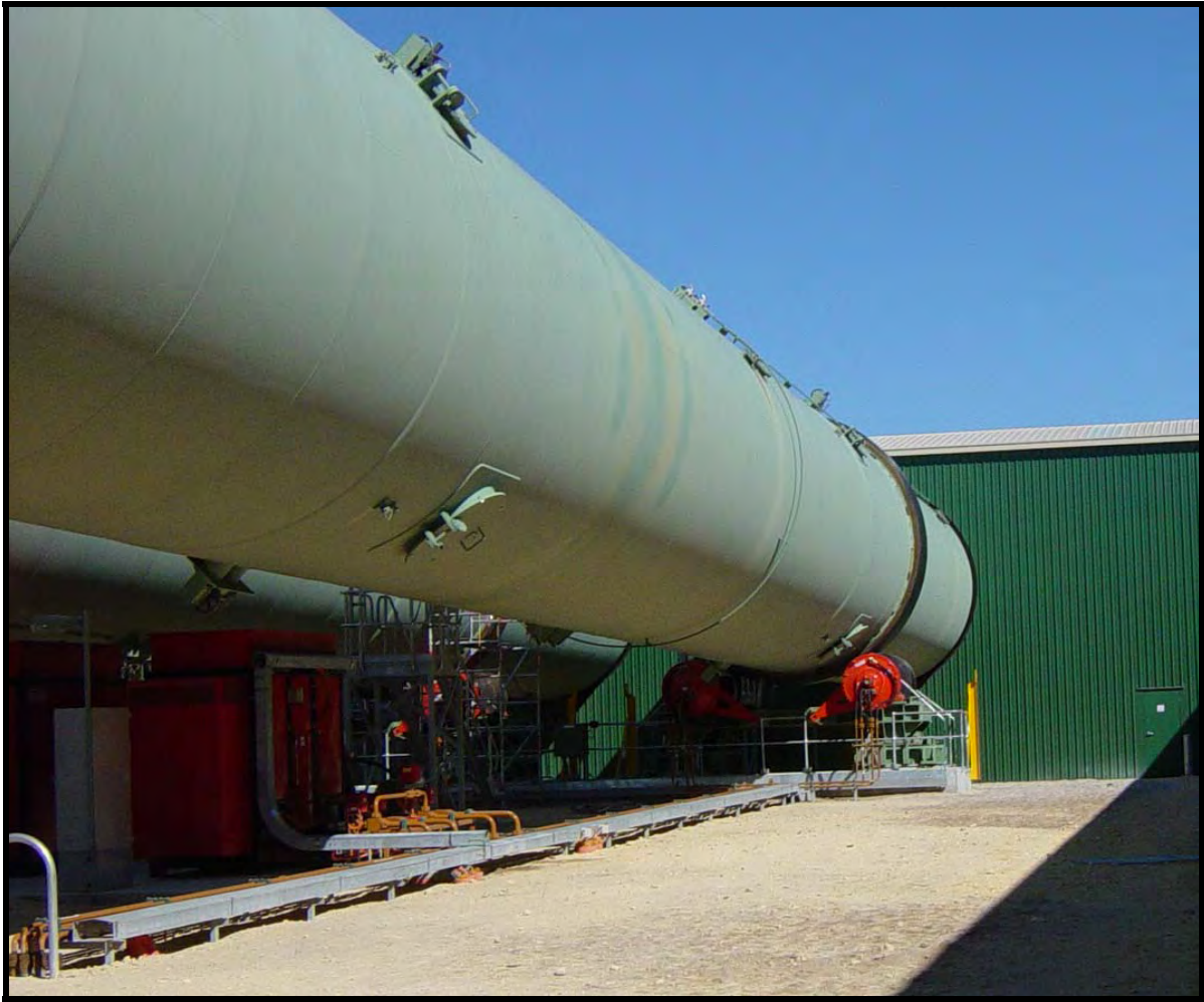
Figure VIII-8. Example of Eweson drum design (Western Australia)
