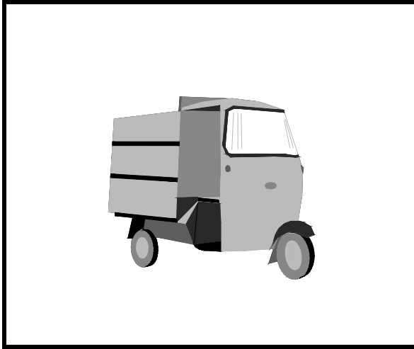
Figure IV-15. Light motorised tricycle (about 2 m 3 capacity)
