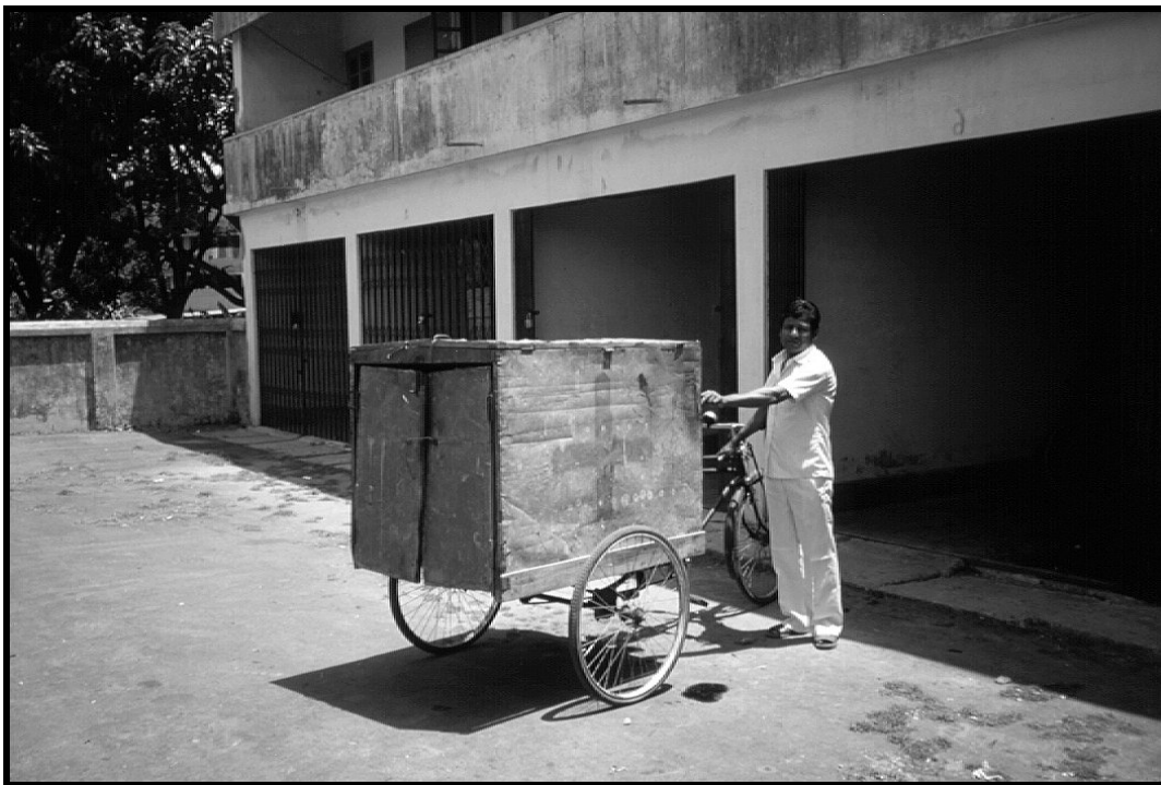
Figure IV-13. Modified pedal tricycle used for waste collection
