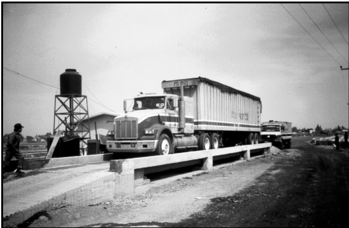
Figure IV-25. Typical open-top trailer used in Mexico City, Mexico
