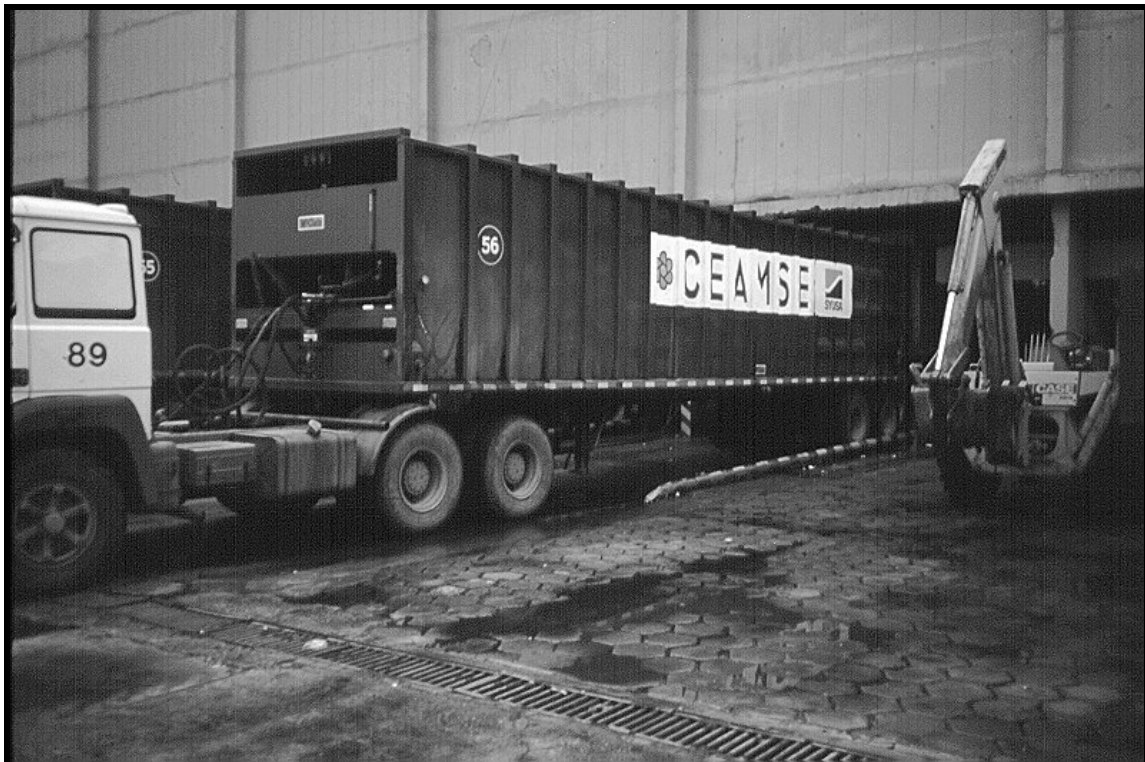
Figure IV-24. Transfer trailer being loaded by a compactor
