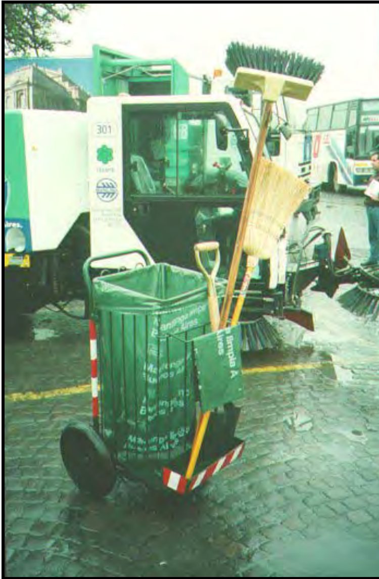
Figure IV-11. One-bin handcart (100- to 200-L capacity)
